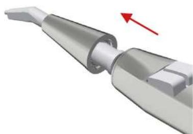
Withdraw the nozzle retainer.
