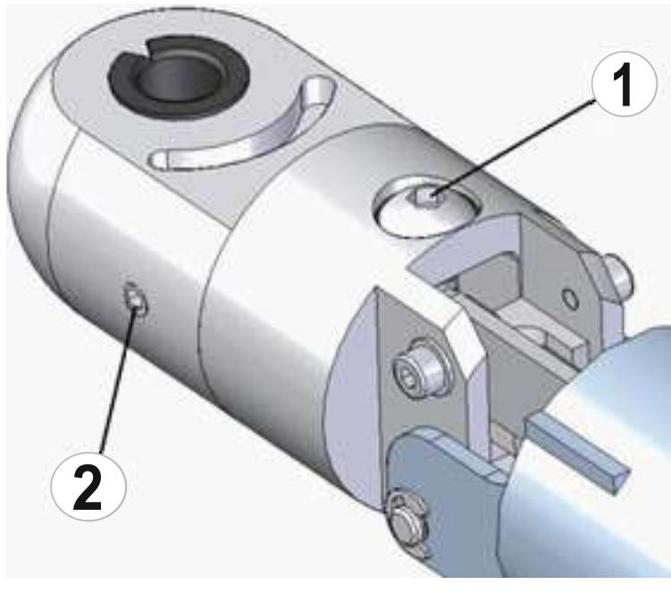
With the adjusting screw, the tray can be aligned in its radially horizontal position.
