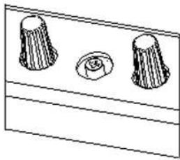
Below the doctor's device, the spray intensity can be regulated. The valve groups (3-fold) for an instrument are arranged according to the order of the instruments in the instrument holders.
