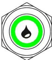
Intensive flushing is activated by a double click on the push-button. The WSU button lights up permanently blue during the phase of double dosage. When the rinsing is activated, the WSU button flashes green-blue. When the rinsing process is finished, the button lights up permanently green. The return to normal operation is indicated on the display.
